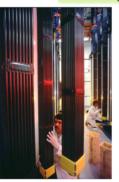
Pellets are placed in fuel rods rods are combined into fuel assemblies
