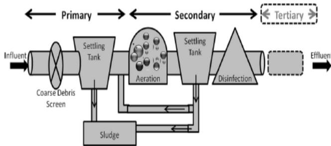
Figure 2: Schematic of a typical municipal facility indicating stages of processing. Tertiary treatment is optional and, if present, will vary between facilities. Coarse debris screening (identified here as part of primary treatment) can also be considered preliminary treatment (Mason et al. 2016, 2).
