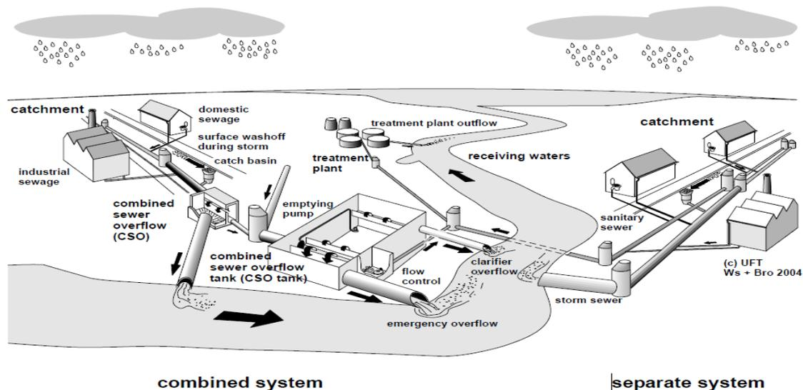
**Figure 1.** Traditional combined (left) and separate (right) sewer systems.
