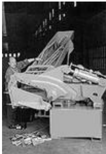
This particular type of shear is an alligator shear and would be the most logical choice for destroying weapons.
