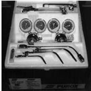
Oxy-Acetylene Torch with Accessories
